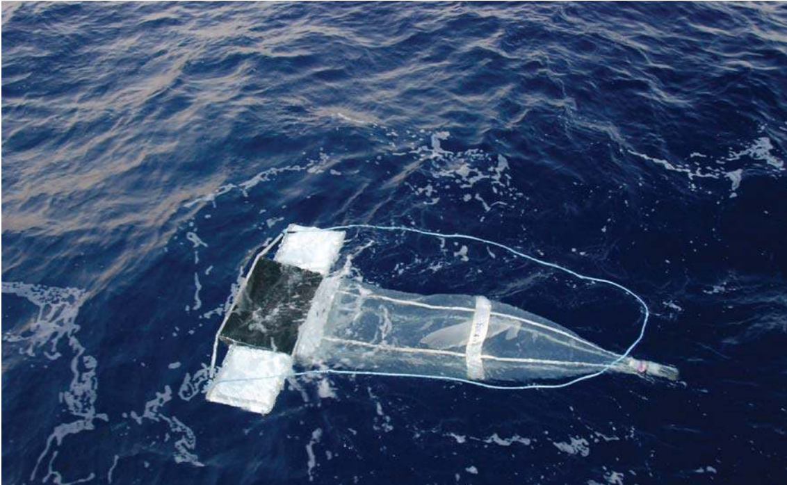
Towed Manta trawl for sampling the ocean surface for floating microplastics – (NOAA News Archive)
